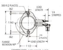
STRIPPED ENDS, quick connect, eyelets and other terminal configurations available
